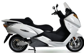
Fig. 14. Battery scooter (Vectrix Corp, 2010) Battery: Li: LiFePO 4 , 30Ah capacity
