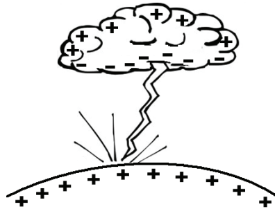
Fig. 1. Thundercloud charge distribution of lightning between cloud and ground
