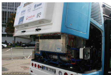
Fig. 2. Detail on fuel cells, the ESS is composed of Li-ion battery and supercapacitors (TriHyBus.cz, 2008)
