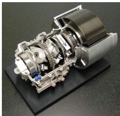
Fig. 31. The original CVT based Formula One KERS (Flybrid Systems, 2010)
